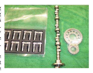
Roller rockers introduce a bearing for each rocker instead of a metal-to-metal lubrication point of 1960s engine technology. Like the hydraulic roller camshaft, it improves efficiency by reducing internal friction and prolongs the life of the engine by eliminating another metal-to-metal wear point.
