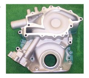
An improved design makes the high-capacity water pump able to move much more coolant than the OEM Buick water pump of the 1960s.
